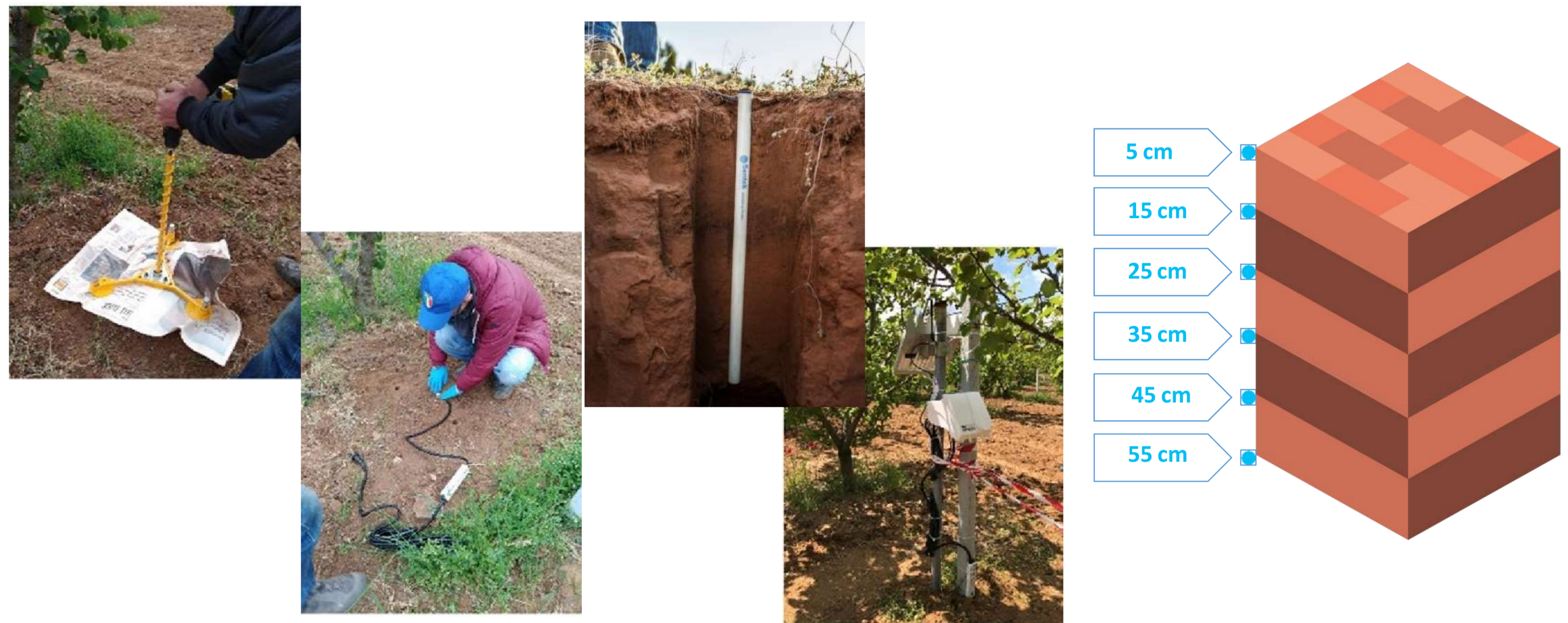
Fig. 1. Drill&Drop automated sensors installed in an Apricot farm, Southern Italy.
